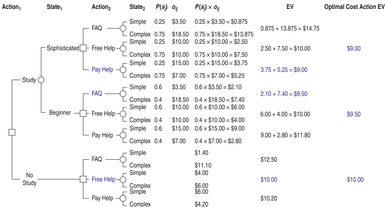
Figure 24.3 A decision tree including a customer history study. For each decision node under each circumstance, the optimal (in this example, lowest cost) alternative is indicated in color, and the corresponding consequence is assigned as the expected value for that alternative. EV's for the No Study branch are from Figure 24.2.
